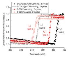
Fig. 12 Thermal dependence of the normalized optical reflectivity recorded at 2 K min<sup>-1</sup> on both SCO-2@MCM (black curves) and SCO-2 prepared as nanoparticles (red curves) using the reverse micelle method. The transition temperatures in the warming and cooling modes are given.
