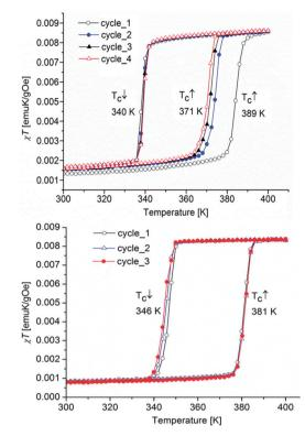
Fig. 10 Temperature-variable magnetic curves for SCO-1@MCM (top) and SCO-2@MCM (bottom).
