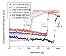
Fig. 11 Thermal dependence of the normalized optical reflectivity of SCO-1@MCM at a scan rate of 2 K min<sup>-1</sup>. The transition temperatures recorded in warming and cooling modes are indicated
