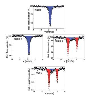
Fig. 7 Selected <sup>57</sup>Fe Mössbauer spectra of SCO-1@MCM; blue and red colors correspond to LS and HS doublets, respectively
