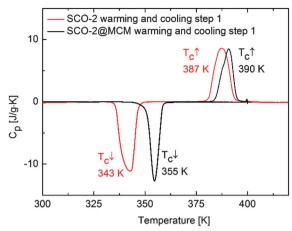
Fig. 13 Heat capacity versus temperature for SCO-2 and SCO-2@MCM recorded by differential scanning calorimetry at 10 K min<sup>-1</sup>.
