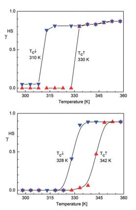
Temperature dependence of the HS molar fraction ( $\gamma^{HS}$ ) deduced from <sup>57</sup>Fe Mössbauer spectroscopy over the temperature range 298–360 K for SCO-1@MCM (top) and for SCO-2@MCM (bottom).
