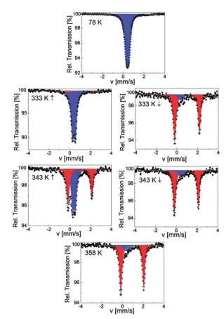
Fig. 9 Selected <sup>57</sup>Fe Mössbauer spectra of SCO-2@MCM; red and blue colors correspond to HS and LS doublets, respectively.
