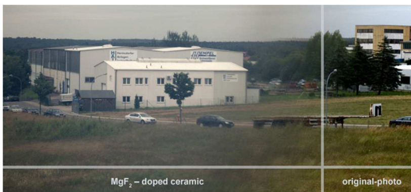
Figure 17: Picture taken wherein the left side of the camera lens (2/3 of the image) is covered by the “new transparent ceramic” disc whereas the right side shows the original photo.
