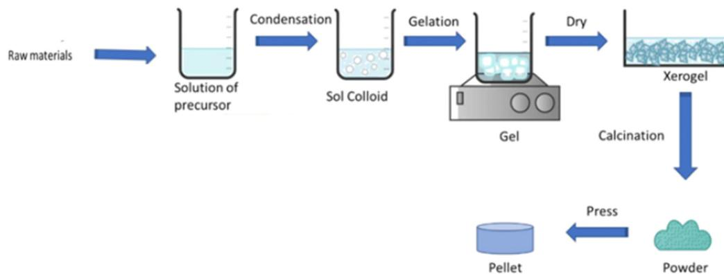
Fig. 6 Schematic view of the sol-gel method.<sup>189</sup> Reprinted with permission from ref. 189. Copyright ©2020, Elsevier Inc.
