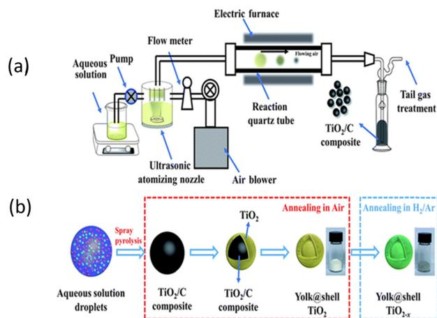
Fig. 4 Schematic diagram of (a) ultrasonic spray pyrolysis process and (b) mechanism of yolk@shell-structured  $\text{TiO}_{2-x}$  prepared using the ultrasonic pyrolysis method. Reprinted with permission from ref. 163. Copyright: 2019, the Royal Society of Chemistry.
