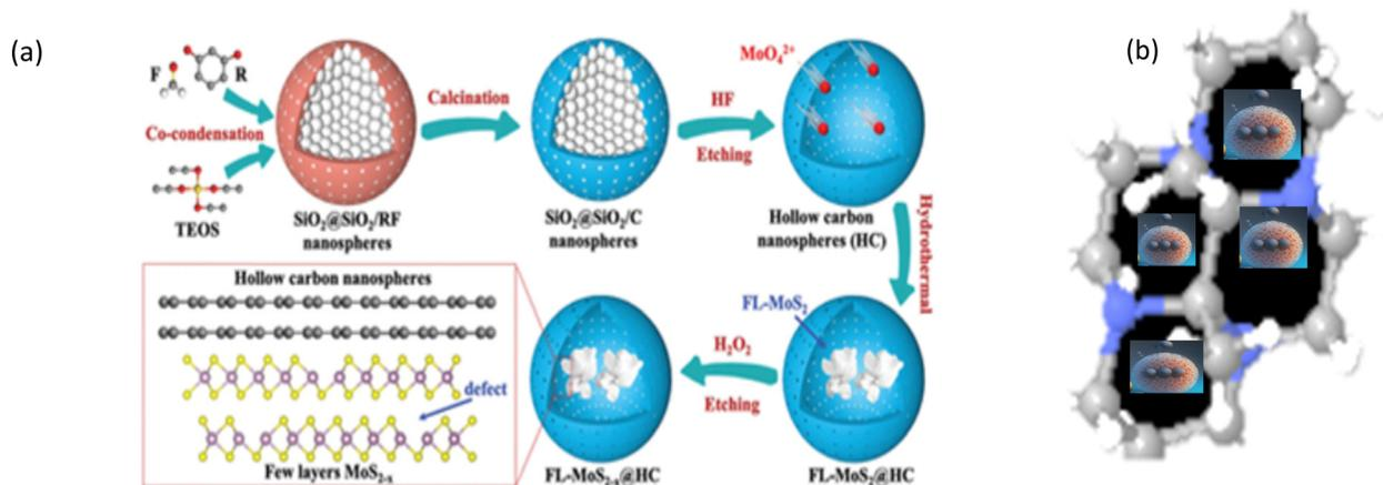
Fig. 5 (a) Illustration of the preparation process of the FL-MoS<sub>2-x</sub>@HC matrix. (b) Molecular assembly into the molecular porous template. Reprinted with permission from ref. 176. ©2021, Wiley-VCH GmbH.
