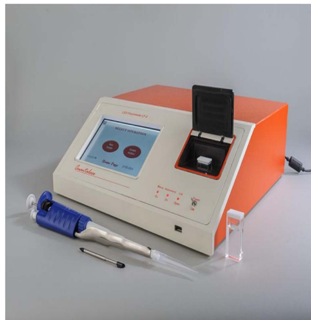
Fig. 2 LED fluorimeter (model LF-2) (Quantalase, India).
