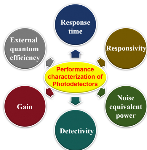
Fig. 6 Performance characterization of photodetectors.
