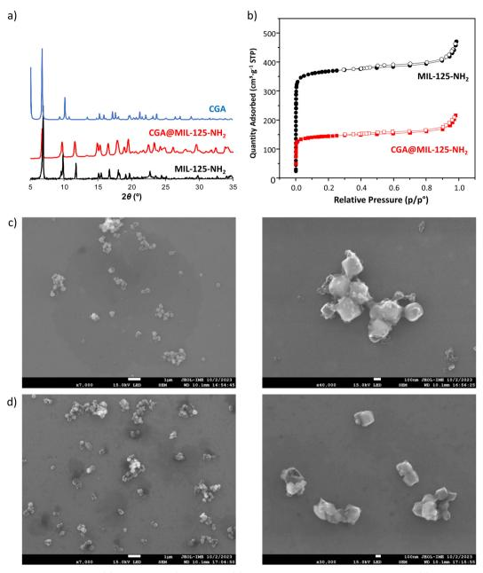
Fig. 1 (a) XRPD patterns of pristine and CGA loaded MIL-125-NH<sub>2</sub>. Free CGA XRPD pattern was added for comparison. (b) N<sub>2</sub> sorption isotherms (77 K) for MIL-125-NH<sub>2</sub> before (black, circles), and after (red, squares) the CGA loading. Empty symbols denote desorption. FE-SEM images of (c) MIL-125-NH<sub>2</sub> and (d) CGA@MIL-125-NH<sub>2</sub>. No significant differences after the CGA encapsulation are observed in the cubic shaped particles.
