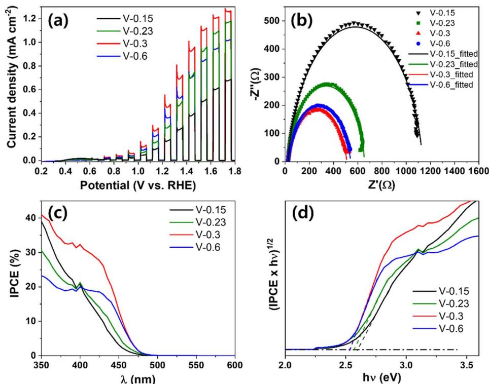
Fig. 8 Photoelectrochemical performances of  $\text{BiVO}_4/\text{WO}_3$  photoanodes depending on V concentrations of 0.15, 0.23, 0.3, and 0.6 M of the  $\text{BiVO}_4$  precursor; (a) photocurrent densities by linear sweep voltammetry, (b) Nyquist plots, (c) IPCE spectra, and (d) bandgap evaluated by IPCE measurement.
