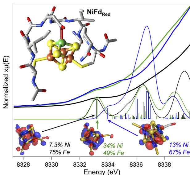
Fig. 7 Experimental pre-edge Ni K-edge XANES spectra of NiFd<sub>red</sub> (green), NiFd<sub>ox</sub> (black), and NiFd–CO (blue) with calculated TD-DFT contributions using the DFT geometry-optimized structures of the NiFd species (inset). Dominant contributing orbital to the indicated transition for each species shown at an isosurface value of 0.03 with distribution over Ni and the Fe atoms indicated.
