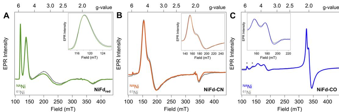
Fig. 2 CW X-band EPR spectra ( $\nu = 9.37$  GHz,  $P_{\mu\text{W}} = 20$  mW,  $T = 8.0$  K) of natural abundance (colored traces) and  $^{61}\text{Ni}$ -isotopically labelled (gray traces) samples of (A) NiFd<sub>red</sub>, (B) NiFd-CN, and (C) NiFd-CO. (Insets) Zoomed in views of low-field turning points highlight  $^{61}\text{Ni}$ -induced broadening. \* indicates residual NiFd<sub>red</sub> that remains after exposure to CO.
