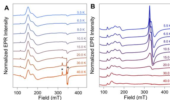
Fig. 3 CW EPR spectra ( $\nu = 9.37$  GHz,  $P_{\mu\text{W}} = 20$  mW) of (A) NiFd-CN and (B) NiFd-CO at the indicated temperatures. Spectra were normalized to temperature using a standard Curie dependence [ $I \propto T$ ]. \* denotes small ( $<5\%$ ) amount of contaminating  $S = 1/2$   $[\text{Fe}_4\text{S}_4]\text{-CN Fd}$ .
