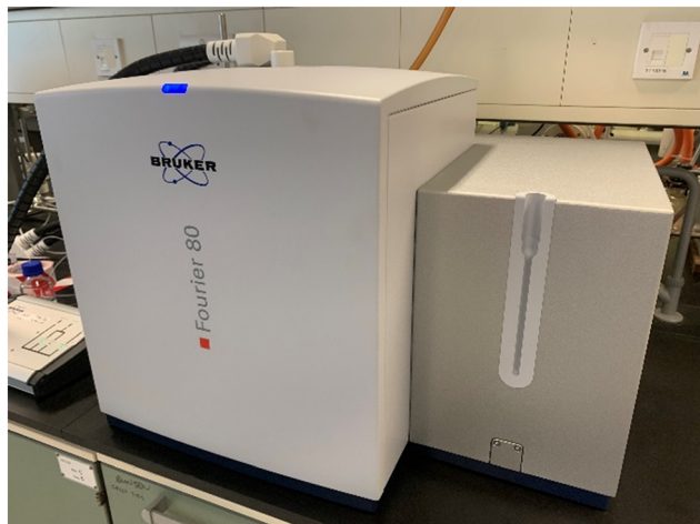
Fig. 5 Image of Bruker 80 MHz benchtop NMR spectrometer.
