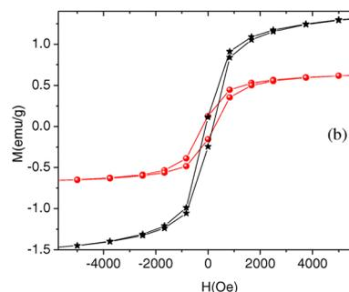
Fig. 2 Room temperature magnetization curves of PANI/Se<sub>0.95</sub>Fe<sub>0.05</sub> (5 wt% in black and 10 wt% in red) nanocomposites. [Reproduced from ref. 24, with permission from Springer, Copyright 2019.]
