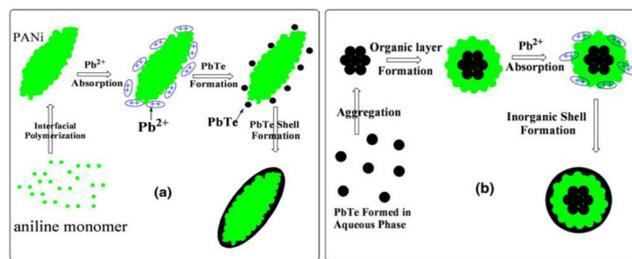
**Fig. 12** Illustration of the growth mechanism for (a) PANI/PbTe core-shell structure and (b) PbTe/PANI/PbTe three-layer nanostructure. [Reproduced from ref. 44, with permission from Springer, Copyright 2011.]
