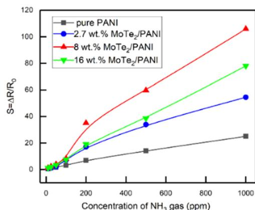
Fig. 17 Comparison of the sensing response of composites as a function of NH<sub>3</sub> gas concentration in the lab-environment. [Reproduced from ref. 84, with permission from MDPI, Copyright 2022.]
