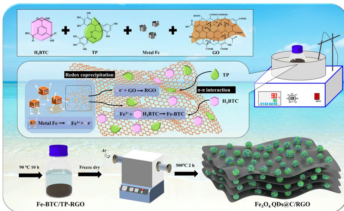
Scheme 1 Schematic illustration for the synthesis of the Fe<sub>3</sub>O<sub>4</sub> QDs@C/RGO sample.
