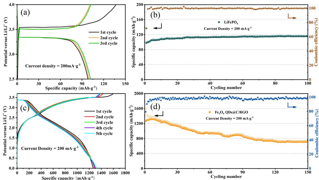
**Fig. 8** Charge and discharge voltage profile (a) and cycling performance (b) of a commercial  $\text{LiFePO}_4$  cathode at  $200 \text{ mA g}^{-1}$  in half cells. Charge and discharge voltage profile (c) and cycling performance (d) of the  $\text{Fe}_3\text{O}_4$  QDs@C/RGO sample in  $\text{Fe}_3\text{O}_4$  QDs@C/RGO// $\text{LiFePO}_4$  full cells at  $200 \text{ mA g}^{-1}$ .
