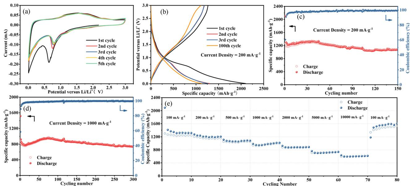
Fig. 4 The CV curves for the initial 5 cycles (a), and charge and discharge voltage profile (b) of the  $\text{Fe}_3\text{O}_4$  QDs@C/RGO composite. Cycling performance under a low current density of  $200 \text{ mA g}^{-1}$  (c), long-term lithium-ion storage capability under a current density of  $1000 \text{ mA g}^{-1}$  (d), and rate capability (e) of the  $\text{Fe}_3\text{O}_4$  QDs@C/RGO composite.
