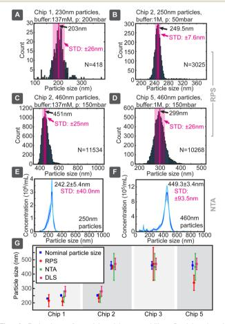
Fig. 4 Evaluation of particle sizing capability. Particle size is calculated analytically from device geometry without calibration. (A-D) Examples of obtained distributions of particle sizes with mean value and standard deviation. (E and F) Comparison with NTA. (G) Comparison of different chips used to measure particle sizes, nominal values and measurements with commercial NTA and DLS systems (error bars indicate one standard deviation, values for RPS are based on N = 7 devices).
