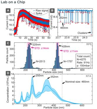
distribution measurement and concentration polydisperse samples represented by mixture of 252 nm and 460 nm particles in respective concentrations of  $5.7 \times 10^9$  and  $2.9 \times 10^9$ particles per mL. (A) Raw measured signal (blue) with detected particles indicated with red. (B) Same in enlarged scale. (C) Histograms of populations of spikes corresponding to both sizes of particles, while (D) shows NTA measurement of mixture of same particles (108 particles per mL each).
