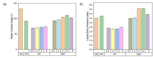
Fig. 5 a) Water CA and b) LEP of fabricated PVDF-clay membranes. Error bars represent standard deviations from three samples.
