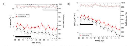
Fig. 7 Long-term stability test of commercial PVDF (black lines) and PVDF-OMT4 wt% (red lines) membranes for permeate flux and salt rejection in presence of only a) NaCl and b) NaCl with HA to promote scaling phenomena. Full and empty symbols represent the membrane flux (kg m $^{-2}$  h $^{-1}$ ) and salt rejection (%), respectively. Error bars represent standard deviations from three samples (or five in the case of the porosity).
