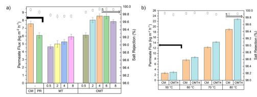
Fig. 6 Average total permeate flux and salt rejection of the prepared PVDF-clay membranes at a) 60 °C and at b) different feed temperatures for commercial PVDF and the OMT 4 wt% membranes. Columns: permeate flux (kg m $^{-2}$  h $^{-1}$ ), and square symbols  $\Box$ : salt rejection (%). Error bars represent standard deviations from three samples.
