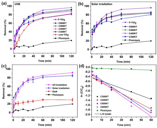
Fig. 4 Degradation of TET under (a) UVB and (b) solar irradiation using com-TiO2, P-TiO2, C300KT, C400KT, C500KT, and C600KT along with the control photolysis experiment (no catalyst present), (c) comparison of the efficiency of C600KT with the dark experiment, and (d) Langmuir-Hinshelwood kinetic fits for all measurements. Some of the error bars are small and directly on the plot symbols, the same figure only showing the error bars can be found in the Fig. S3.†
