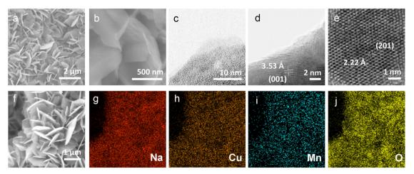
Fig. 2 (a) Low-, (b) high-resolution SEM images of the morphology of the NCMO. (c) low-, (d) high-resolution and (e) atomic resolution STEM images for surface structures of NCMO. (f)-(j) EDS mapping images of NCMO show that Na, Cu, Mn, and O elements are uniformly distributed.
