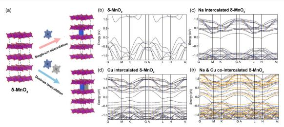
Fig. 1 (a) Ion intercalation strategy for high performance  $\delta$ -MnO<sub>2</sub> cathode materials and band structures of (b)  $\delta$ -MnO<sub>2</sub>, (c) Na intercalated  $\delta$ -MnO<sub>2</sub>, (d) Cu intercalated  $\delta$ -MnO<sub>2</sub> and (e) Na & Cu co-intercalated  $\delta$ -MnO<sub>2</sub> based on DFT modelling
