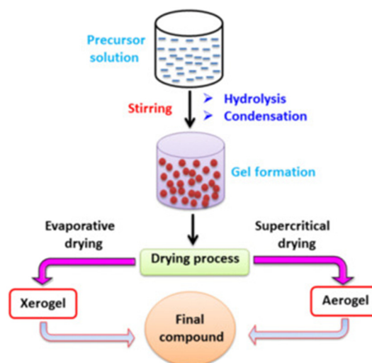
Fig. 14 The scheme process of the sol-gel method. Reproduced from ref. 153 with permission from Journal of Environmental Chemical Engineering, copyright 2021.
