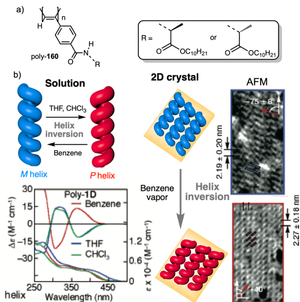
Fig. 78 (a) Chemical structure of poly-L/D-160. (b) Schematic representation of poly-D-158 and its macromolecular helicity inversion in solution and in 2D crystal state. Reproduced from ref. 372 with permission from the American Chemical Society, copyright 2006.
