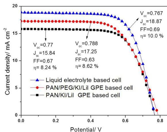
Fig. 8 Photo-current density–voltage characteristics ( $J$ – $V$ ) of DSSCs based on liquid electrolyte, PAN/LiI/KI and PAN-PEG/LiI/KI blended PGEs using an illuminated light intensity of 100  $\text{mW cm}^{-2}$ .
