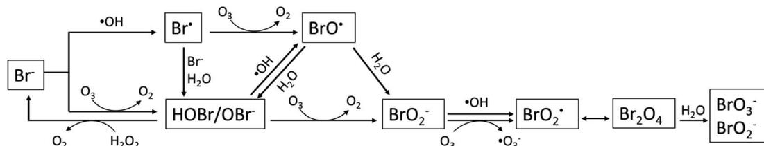
Fig. 1 Reaction pathways for bromate formation during ozone-based AOPs (adapted from Fischbacher *et al.*, 2015;<sup>19</sup> Von Gunten and Hoigne, 1994;<sup>10</sup> von Gunten and Oliveras, 1998.<sup>11</sup>
