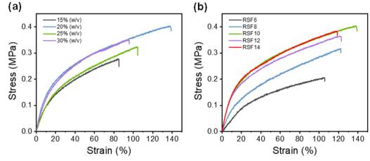
Fig. 3 Typical stress-strain curves of wet RSF films prepared at (a) different  $(NH_4)_2SO_4$  concentrations ranging from 15% (w/v) to 30% (w/v) and (b) different SF concentrations ranging from 6 wt% to 14 wt% (20% (w/v)  $(NH_4)_2SO_4$  solution).
