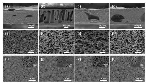
Fig. 2 SEM images of the cross sections (a-h) and surface (i-l) of RSF films prepared from 15% (w/v) (NH<sub>4</sub>)<sub>2</sub>SO<sub>4</sub> solution (a, e and i), from 30% (w/v) (NH<sub>4</sub>)<sub>2</sub>SO<sub>4</sub> solution (b, f and j), and from 6 wt% SF concentrations (c, g and k) and 10 wt% SF concentrations (d, h and l) (20% (w/v) (NH<sub>4</sub>)<sub>2</sub>SO<sub>4</sub>.
