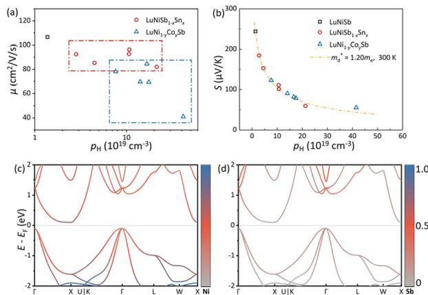
Fig. 6 (a)  $\mu_H$  as a function of  $\rho_H$  and (b) the Pisarenko curves with  $m_d^* \approx 1.2 m_e$  for  $\text{LuNiSb}_{1-x}\text{Sn}_x$  and  $\text{LuNi}_{1-y}\text{Co}_y\text{Sb}$  at room temperature. The projected band structure of (c) Ni and (d) Sb for  $\text{LuNiSb}$ .
