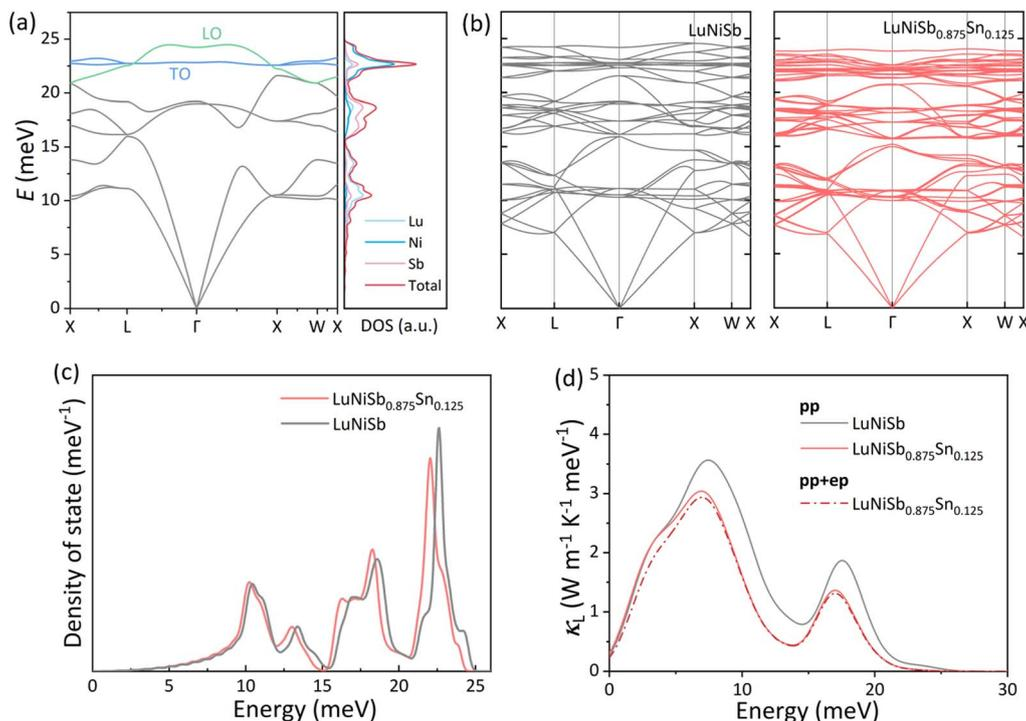
Fig. 3 (a) Calculated phonon dispersion of LuNiSb with total and partial DOS in a single cell. (b) Phonon dispersion of LuNiSb and LuNiSb<sub>0.875</sub>Sn<sub>0.125</sub> in a  $2 \times 2 \times 2$  supercell. (c) Energy-dependent total DOS and (d) room temperature  $\kappa_L$  of LuNiSb and LuNiSb<sub>0.875</sub>Sn<sub>0.125</sub>, where the solid lines were calculated only considering the p–p scattering event and the dotted line applies for both p–p and e–p scattering events.
