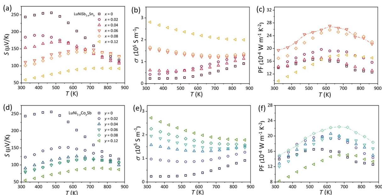
Fig. 5 Temperature-dependent (a and d)  $S$ , (b and e)  $\sigma$ , and (c and f) PF for LuNiSb<sub>1-x</sub>Sn<sub>x</sub> and LuNi<sub>1-y</sub>Co<sub>y</sub>Sb, respectively.
