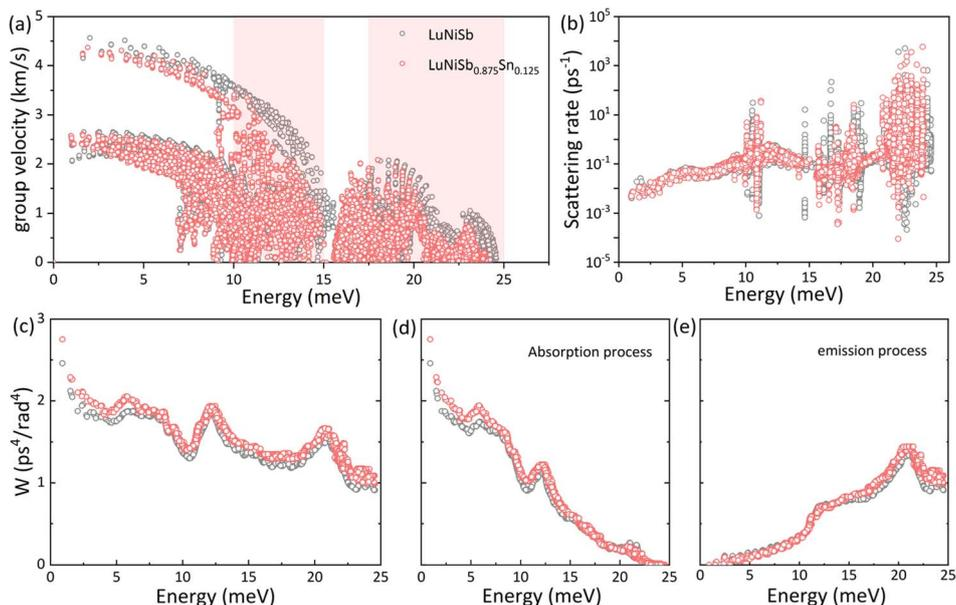
Fig. 4 Calculated group velocity (a) and scattering rate (b) versus the energy of phonon modes for LuNiSb and LuNiSb<sub>0.875</sub>Sn<sub>0.125</sub>. Energy dependence of p-p scattering phase space (c), the absorption process (d) and emission process (e).
