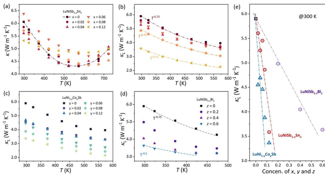
Fig. 2 Temperature dependence of the  $\kappa$  (a) and  $\kappa_L$  (b) for  $\text{LuNiSb}_{1-x}\text{Sn}_x$ . The temperature-dependent  $\kappa_L$  of (c)  $\text{LuNi}_{1-y}\text{Co}_y\text{Sb}$  and (d)  $\text{LuNiSb}_{1-z}\text{Bi}_z$ . (e) Nominal doping of alloying concentration dependence of  $\kappa_L$  for  $\text{LuNiSb}_{1-x}\text{Sn}_x$ ,  $\text{LuNi}_{1-y}\text{Co}_y\text{Sb}$  and  $\text{LuNiSb}_{1-z}\text{Bi}_z$ .
