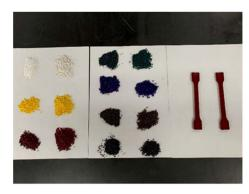
Fig. 23 Biomass biodegradable color masterbatch.
