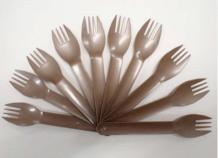
Fig. 42 100% biomass biodegradable resin pellet (Left) and forks (Right) made from Sargassum waste
