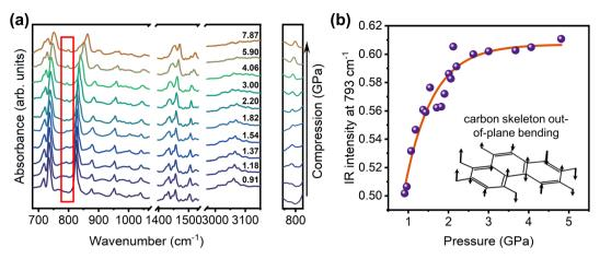
Fig. 2 (a) In situ IR spectra of the phenanthrene crystal upon compression. (b) The pressure-dependent IR absorption intensities around 793 cm<sup>-1</sup> and the schematic diagram of the corresponding vibrational mode. The relevant vibrations are marked in the diagrams (a).
