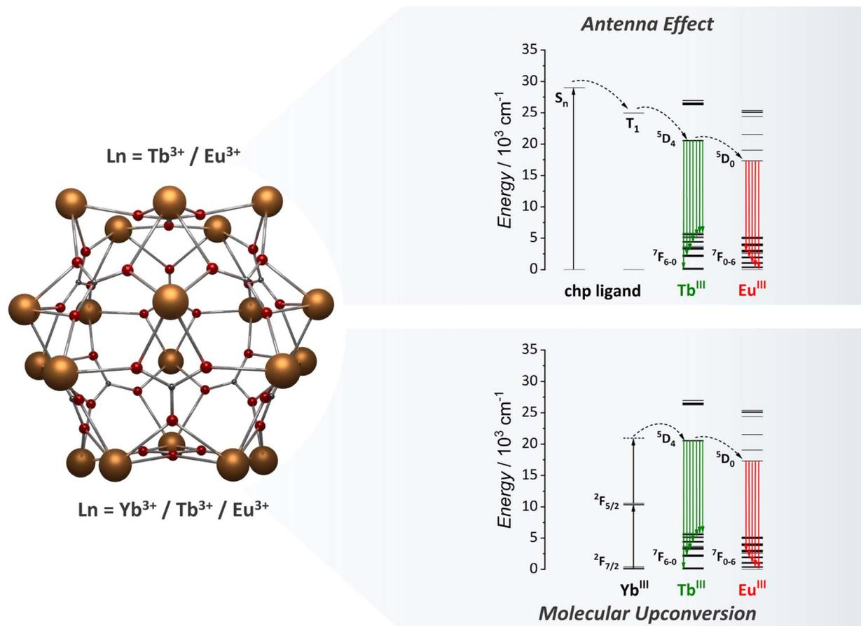
Fig. 7 Metal core structure of the  $\{Ln_{20}\}$  MCAs (CCDC number: 2023766)<sup>81</sup> and the energy transfer mechanism for antenna effect and UC emissions.<sup>81,95</sup> Colour code: Dark orange:  $Ln^{3+}$ ; grey: carbon; red: oxygen. Hydrogen atoms were omitted in the structure for clarity.
