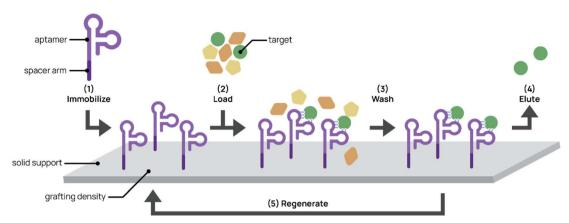
Fig. 5 Aptamers for affinity chromatography. (1) Aptamers designed with spacer arms are immobilized onto a solid support. (2) Mixed input is loaded onto the platform and aptamer captures the target. (3) The platform is washed to remove non-targets. (4) The target is eluted from the support. (5) In some cases, the platform can be regenerated for repeated use.
