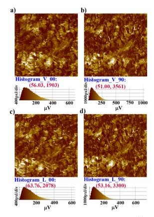
Fig. 4 PFM amplitude image of a crystalline thin film of 1: (a) and (b) vertical and (c) and (d) lateral amplitude images collected by scanning the  $\it X$  and  $\it Y$  directions; the indication of 0 and 90 is relative. The corresponding histograms show that the maximum number of pixels have the most occurring amplitude value of deformation (in  $\mu V$ ).
