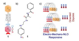
Scheme 1 (a) Schematic representation of molecule 1 with its important structural components: aromatic unit- $\pi_a$ , dipolar unit- $\pi_b$  and the chiral spacer; (b) molecular structure of 1; (c) supramolecular assembly of 1 to form highly oriented dipoles to function as an electromechano and NLO responsive single-component material.
