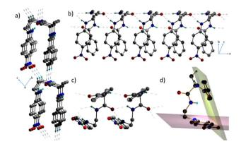
Fig. 1 POV-ray representation of the single-crystal structure of 1 showing: (a) its folded structure and ability to form highly oriented dipoles utilizing H-bonding interactions; (b) and (c) various intermolecular non-covalent H-bonding interactions; (d) angle subtended by the two  $\pi$ -units. The atoms C, O, N and H are represented in grey, red, blue and light cyan, respectively.
