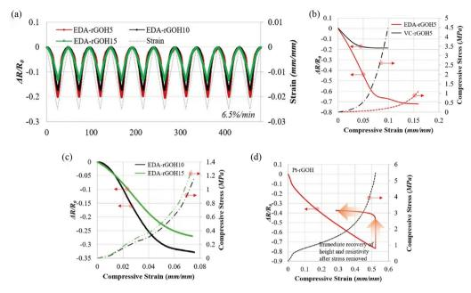
Fig. 9 Piezoresistive properties of graphene oxide hydrogel (GOH) under different modification conditions. (a) Cyclic compressive strain-induced resistance changes of different concentrations of GOH at strain frequencies of 6.5% min<sup>-1</sup>. Piezoresistive behavior and s-s curve of (b) EDA-rGOH5 and VC-rGOH5, (c) EDA-rGOH10 and EDA-rGOH15, and (d) Pt-rGOH under static compressive strain with a strain rate of 6.5 cm min<sup>-1</sup>.114
