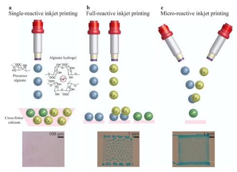
Fig. 16 Illustration of three different reactive inkjet 3D printing strategies. (a) Single-, (b) full-, and (c) microreactive inkjet printing. 197
