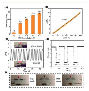
Fig. 4 Testing of the electrical properties of polymer conductive hydrogels. (a) Conductivity of hydrogels with different ANI concentrations. (b) Variation of hydrogel resistance under applied strain ( $\Delta R/R_0$ ). (c) Change in the resistance of the conductive hydrogel during the cyclic test. (d and e) Changes in LED bulb brightness before and after self-healing. 63
