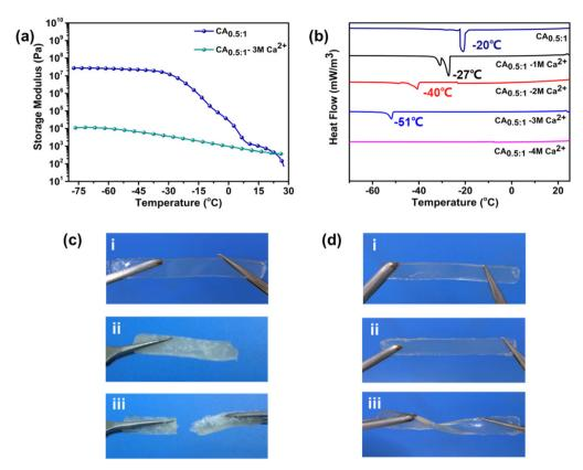
Fig. 5 Antifreezing test of ionic conductive hydrogel. (a) DMA curves of  $CA_{0.5:1}$  and  $CA_{0.5:1}$ -3 M  $Ca^{2+}$  when the temperature changes from 25 to -75 °C, (b) DSC curves of CA<sub>0.5:1</sub> and CA<sub>0.5:1</sub>-Ca<sup>2+</sup> when the temperature changes from 25 to -75 °C, and (c and d) images of CA<sub>0.5:1</sub> and CA<sub>0.5:1</sub>-3 M Ca<sup>2+</sup> bending at -50 °C, respectively.<sup>7</sup>
