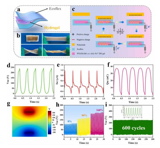
Fig. 11 (a) Structure of PP-TENG. (b) Images of PP-TENG under the different states. (c) Illustration of the power generation mechanism. (d) V<sub>OC</sub>, (e)  $I_{SC}$ , and (f)  $Q_{SC}$  of the PP-TENG. (g) Finite element analysis of PP-TENG output voltage. (h) Open-circuit voltage of the stretchable PP-TENG at different strains. (i) Stability of the PP-TENG under 600 cycles. 139
