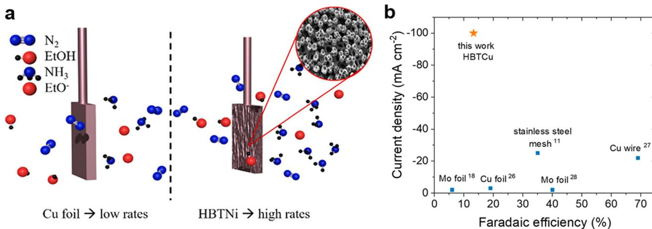
Fig. 6 (a) Illustration of Cu foil and HBT Cu for Li-mediated eN<sub>2</sub>RR; (b) comparison of HBT Cu and previously reported electrode materials in terms of current density and NH<sub>3</sub> FE.<sup>58</sup>
