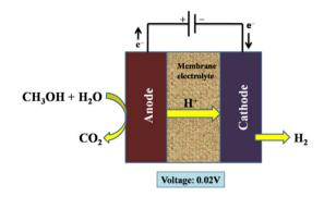
Fig. 24 Electrolysis using organic fuel methanol.
