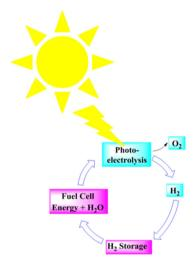
**Fig. 13** A renewable hydrogen cycle. Modified from ref. 209 with permission from Elsevier, copyright 2002.
