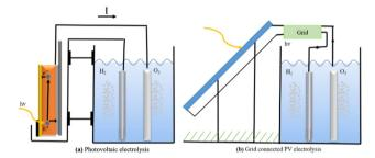
Fig. 18 (a) Photovoltaic electrolysis. (b) Grid-connected PV electrolysis.
