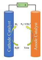
Fig. 26 Electrolysis using organic compound urea.
