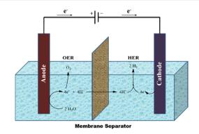
Fig. 3 Electrolysis cell for splitting water. Reproduced from ref. 104 with permission from Nature Publishing Group UK London, copyright 2017.
