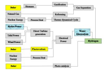
**Fig. 1** The primary energy sources considered and their routes to hydrogen. Reproduced from ref. 10 with permission from Elsevier, copyright 2005.
