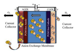
Fig. 12 Working principle of an AEM electrolysis cell.
