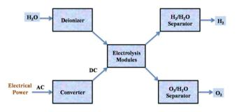
**Fig. 4** Flow diagram of the water electrolysis process. Reproduced from ref. 20 with permission from Elsevier, copyright 2017.
