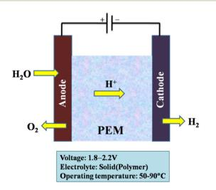
Fig. 10 Illustration of a PEM electrolysis cell.
