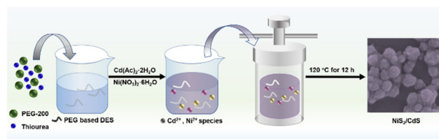
Fig. 1 A schematic illustration of the formation of NiS_2/CdS photocatalyst.
