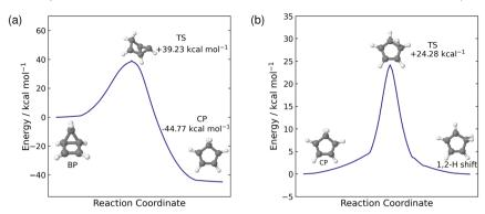
Fig. 7 Intrinsic reaction coordinate (IRC) pathways, computed at the PBE0/def2-TZVP level of theory, from the transition states to each of the minima for both of the reactions that occur on the ground state: the back reaction from BP to CP (a) and the 1,2-hydrogen shift (b). The energies on the plots correspond to energies of the optimised minima and TS geometries at the PBE0/def2-TZVP level and are shown relative to the structure on the left of each of the plots.
