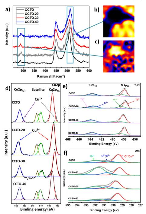
Fig. 4 (a) Raman shifts of the CCTO samples prepared using different PMMA amounts (0, 20, 30, and 40 wt%). (b and c) Raman maps: (b) 510 cm $^{-1}$  (CCTO) and (c) 291 cm $^{-1}$  (CuO). (d-f) High-resolution XPS spectra of (d) Cu  $2p_{3/2}$ , (e) Ti  $2p_{3/2}$ , and 9f) O 1s for the CCTO samples prepared using different PMMA amounts (0, 20, 30, and 40 wt%).
