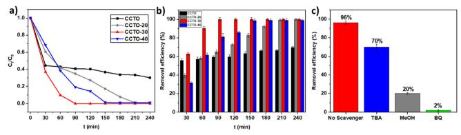
Fig. 7 (a) PCM degradation by electrocatalysis via PMS activation. (b) PCM removal efficiency. (c) Radical scavengers test. TBA: tert-butanol (·OH scavenger); MeOH: methanol (·OH and 'SO scavenger); BQ: p-benzoquinone ('O2 scavenger).
