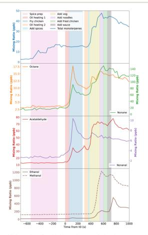
Fig. 2 Mixing ratios of multiple species seen during the average stir-fry experiment, averaged across the two stir-fry repeats.  $t_0$  is the time when oil is added to a hot pan. Shaded areas indicate the different steps of the stir-fry cooking process.
