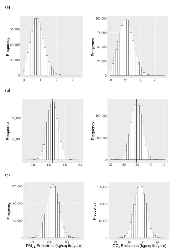
Fig. 2 Particulate matter (PM<sub>2.5</sub>, left) and carbon dioxide (CO<sub>2</sub>, right) annual emission estimate distribution from Monte Carlo samplings for (a) the Xalapán region of Jalapa, (b) the city of Jutiapa, and (c) Guatemala city.
