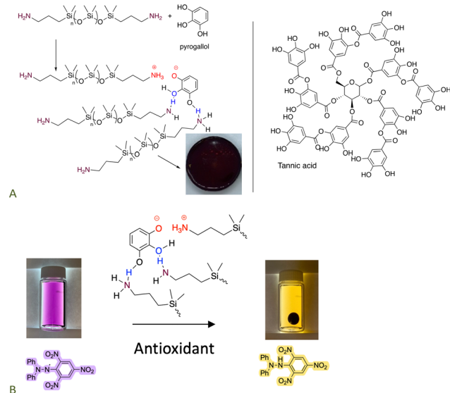
Fig. 13 (A) Formation of elastomers simply by mixing aminosilicones with phenols. (B) Antioxidant activity of the elastomer formed. 70 Photographs from ref. 70 reproduced with permission from the American Chemical Society.
