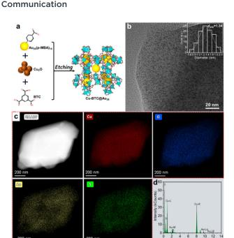
Fig. 1 (a) Schematic illustration of the preparation process of the Au<sub>25</sub>@ Cu-BTC composite. (b) HRTEM image, (c) STEM image and corresponding EDS elemental mapping images and (d) EDS spectrum of Au<sub>25</sub>@Cu-BTC.
