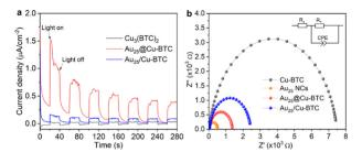
Fig. 3 (a) Photocurrents and (b) Nyquist plots of Cu<sub>3</sub>(BTC)<sub>2</sub>, Au NCs, Au<sub>25</sub>@Cu-BTC and Au<sub>25</sub>/Cu-BTC. The inset in (b) is the equivalent circuit for fitting.
