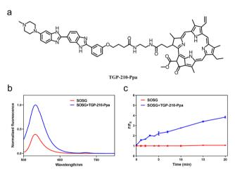
Fig. 1 (a) Chemical structure of TGP-210-Ppa. (b) Fluorescence spectra of **TGP-210-Ppa** after irradiation with 670 nm light (70 mW cm<sup>-2</sup>) for 5 min. (c) The increase of SOSG fluorescence at 530 nm after incubation with TGP-210-Ppa and irradiation by 670 nm light (70 mW cm<sup>-2</sup>) for 0–20 min.  $\lambda_{\rm ex}$  = 488 nm. Data are shown as mean  $\pm$  SEM (n = 3).
