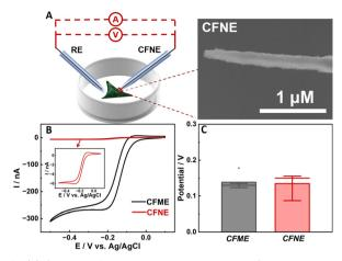
Fig. 1 (A) Scheme of the cell detection with the CFNE by using the amperometric method and open-circuit potential. Inset: SEM image of the bare CFNE. Cyclic voltammograms (B) and statistics potential response (C) obtained at the bare carbon fiber microelectrode (black) and carbon fiber nanoelectrode (red) in HEPES buffer containing 1 mM Ru(NH<sub>3</sub>)<sub>6</sub><sup>3+</sup>.
