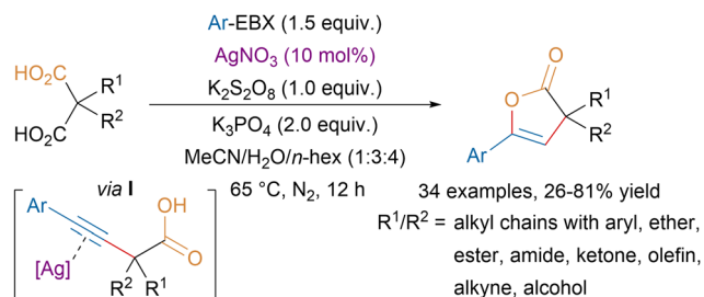
Scheme 34 Ag-catalyzed monodecarboxylative alkylation–lactonization of malonic acid derivatives.
