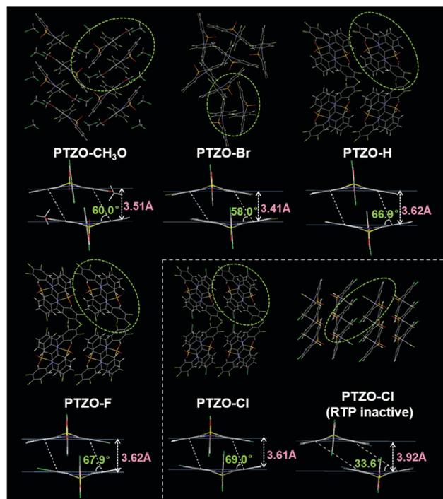
Fig. 3 Single-crystal structures of the five target compounds. Entire and local packing modes of the crystals for PTZO-CH<sub>3</sub>O, PTZO-Br, PTZO-H, PTZO-F, PTZO-Cl and PTZO-Cl (RTP inactive). The local packing pictures are selected from the parts in cycles of corresponding entire ones, in which the plane–plane distances and the slant angles of the involved planes are listed.
