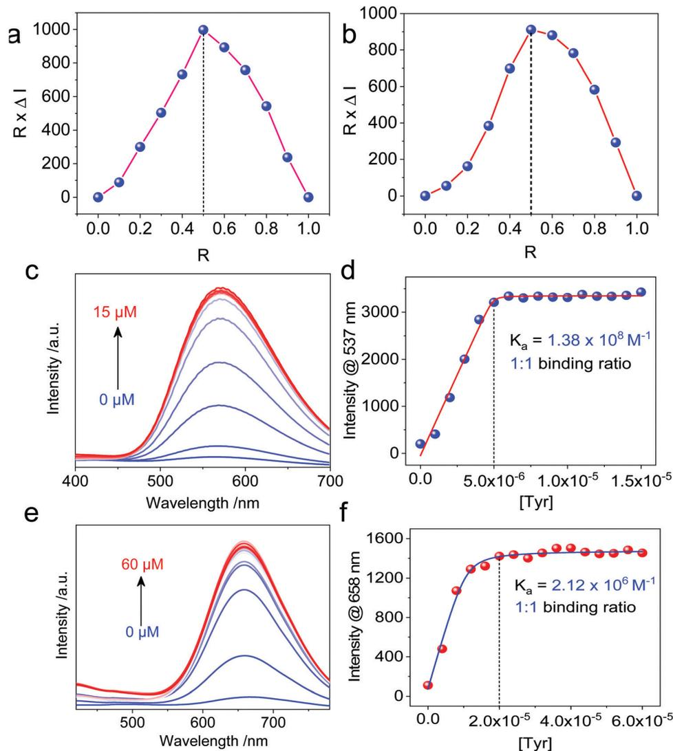
Fig. 3 (a and b) Job's plot curves of **Cycle<sub>1</sub>** and **Cycle<sub>2</sub>**, respectively, with **Tyr** (total concentration = 5  $\mu\text{M}$  in the mixture of acetone and water).  $R$  stands for the molar fraction of **Tyr**. (c and d) **Tyr** concentration-dependent emission spectra of **Cycle<sub>1</sub>** (5  $\mu\text{M}$ ), Ex. = 365 nm. (e and f) **Tyr** concentration-dependent emission spectra of **Cycle<sub>2</sub>** (20  $\mu\text{M}$ ), Ex. = 400 nm.
