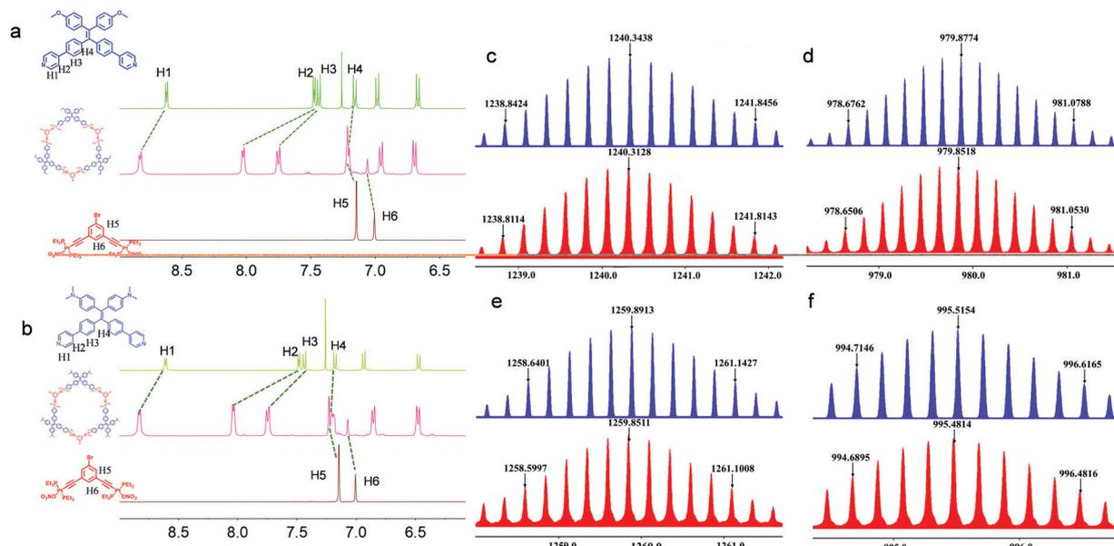
Fig. 1 (a and b) Comparison of <sup>1</sup>H NMR spectra between components in the solvent of acetone-d<sub>6</sub>. (c and d) Electrospray ionization time-of-flight mass spectrometry (ESI-TOF-MS) of **Cycle**<sub>1</sub> with different peaks, where blue and red stand for the calculated and measured spectra, respectively. (e and f) Calculated and measured ESI-TOF-MS peaks of **Cycle**<sub>2</sub>.
