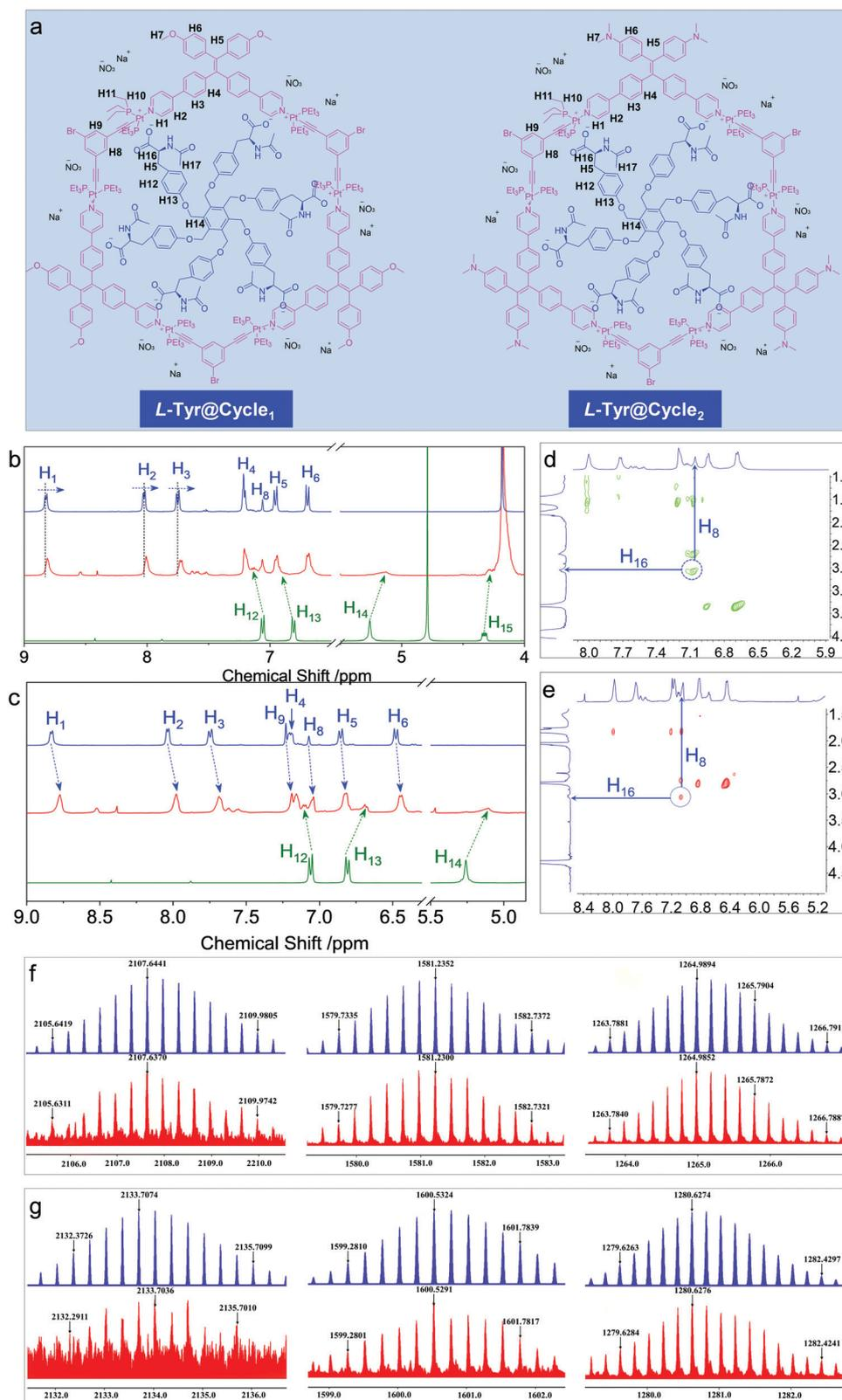
Fig. 5 (a) Proton assignment in the inclusion complexes. (b and c)  $^1\text{H}$  NMR spectra of the **Cycles** and guest molecule in a mixture of acetone- $d_6$  and deuterated water ( $f_w = 60$  vol%). (d and e) The corresponding 2D NOESY spectra. (f and g) ESI-TOF-MS profiles of the **Tyr@Cycle<sub>1</sub>** and **Tyr@Cycle<sub>2</sub>** inclusion complexes.
