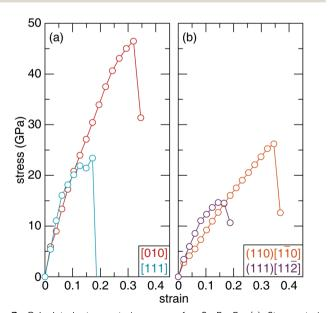
$\label{eq:Fig.7} \begin{tabular}{lll} Fig. 7 & Calculated stress-strain curves for $Sc_2Ru_5B_4$ (a) Stress-strain curves for various crystallographic directions under applied tension. (b) Stress-strain curves for the hardest and softest shear systems. \\ \end{tabular}$
