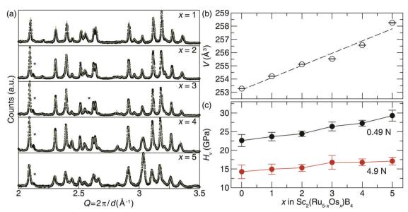
Fig. 3 (a) Powder X-ray diffractograms of the solid solution  $Sc_2(Ru_{5-x}Os_x)B_4$  (x = 1-5). (b) The refined volume determined from Le Bail refinements as a function of x follows Vegard's law. (c) Vickers microindentation ( $H_V$ ) measurements of  $Sc_2(Ru_{5-x}Os_x)B_4$  at low load (0.49 N) and high load (4.9 N).
