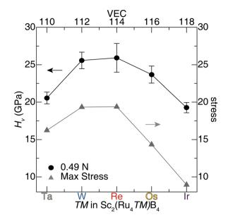
Fig. 8 Vickers hardness and shear stress of softest slip systems in Sc<sub>2</sub>(Ru<sub>4</sub>TM)B<sub>4</sub>.
