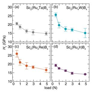
Fig. 6 Vickers microindentation measurements of (a) Sc<sub>2</sub>(Ru<sub>4</sub>Ta)B<sub>4</sub> (b)  $Sc_2(Ru_4W)B_4$ . (c)  $Sc_2(Ru_4Re)B_4$  (d)  $Sc_2(Ru_4Ir)B_4$  from low (0.49 N) load to high load (4.9 N).
