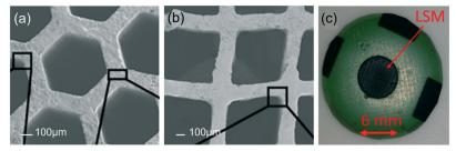
Fig. 22 (a) Hexagonal, and (b) square CGO microstructures of 12 μm depth each, comprising 20 printed layers. Reproduced with permission.<sup>88</sup> (c) photograph of the printed LSM deposited using aqueous-based ink.
