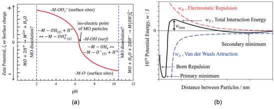
Fig. 10 (a) Schematic pH effect on surface charge and hence zeta potential on metal oxide particles. (b) Schematic effect of inter-particle separation on electrostatic repulsion ( $w_R$ ), van der Waals attraction ( $w_A$ ), and total ( $w_T = w_R + w_A$ ) interaction potentials.
