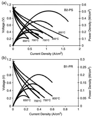
Fig. 25 Effect of current density on cell potential difference for (a) conventional hand-pasted and (b) printed electrode. Reproduced with permission.83
