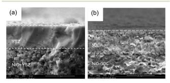
Fig. 23 SEM micrographs showing (a) printed YSZ on Ni-YSZ, and (b) printed SDC on Ni-SDC; post sintering. Reproduced with permission. 90
