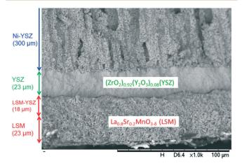
Fig. 16 SEM image of cross-sectional structure of LSM|LSM-YSZ|YSZ| Ni-YSZ SOFC with electrolyte fabricated by inkjet printing.81
