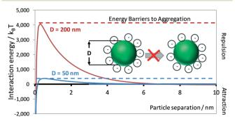
Fig. 11 Effect on interaction energy of particle diameter and separation of YSZ particles in aqueous 10 mol  $\rm m^{-3}$  KCl, stabilised by 0.2 mg  $\rm m^{-2}$  Dispex A40 dispersant.
