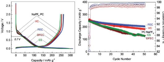
Fig. 3 Cycle performance of hard-carbon anode in 1 mol dm $^{-3}$  NaPF $_6$  in PC-based electrolyte containing 1 vol% of FEC, VC, ES and DFEC additives. <sup>23</sup> Copyright 2016, John Wiley & Sons, Inc.
