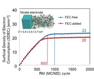
Fig. 5 (a) Charge/discharge curves (1<sup>st</sup> cycle, black line; 30<sup>th</sup> cycle, red line) of carbon-based electrode cycled<sup>23</sup> (Copyright 2016, John Wiley & Sons, Inc)., and (b) the electron consumption used for SEI film formation in NaPF<sub>6</sub> PC/FEC based electrolyte on carbon-based electrode.
