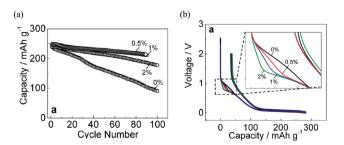
Fig. 7 (a) Capacity retention and (b) initial charge/discharge of hard-carbon electrodes cycled in 1 mol dm $^{-3}$  NaPF $_6$  PC-based electrolyte containing 0, 0.5, 1, and 2 vol% of FEC concentration.  $^{23}$  Copyright 2016, John Wiley & Sons, Inc.
