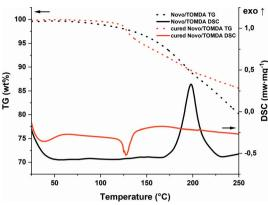
Fig. 6 STA of the TOMDA-formulation (black; TG: dot; DSC: solid) and the photo-DSC cured (red; TG: dot; DSC: solid) sample (90 °C).
