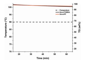
Fig. 7 TGA of the TOMDA-formulation (black) and PF-formulation (red) at 90  $^{\circ}$ C.
