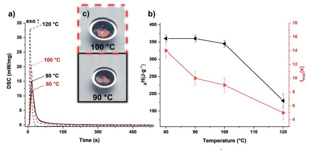
Fig. 5 (a) Photo-DSC of the TOMDA-formulation at 80–120 °C, 2 × 900 s, 320–500 nm, 60 mW cm<sup>-2</sup>. (b) Temperature dependence of photo-DSC results for the TOMDA-formulation: enthalpy change ( $\Delta H$  black) and time until maximal heat is released ( $t_{max}$  red). (c) Cured Samples at 90 & 100 °C.
