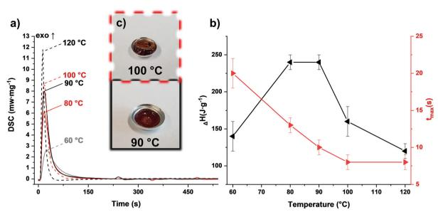
Fig. 3 (a) Photo-DSC of the PF-formulation at 60–120 °C, 2  $\times$  900 s, 320–500 nm, 60 mW cm<sup>-2</sup>. (b) Temperature dependence of photo-DSC results for the PF-formulation: enthalpy change ( $\Delta H$  black) and time until maximal heat is released ( $t_{max}$  red). (c) Cured Samples at 90  $\times$  100 °C.
