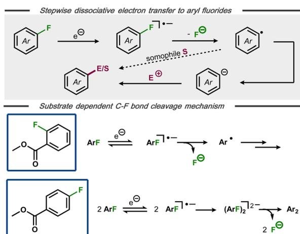
Fig. 5 Top: Mechanism for stepwise defluorination of aryl fluorides. Bottom: Substrate dependent pathways for electroreductive defluorination of methylfluorobenzoates.<sup>34</sup>
