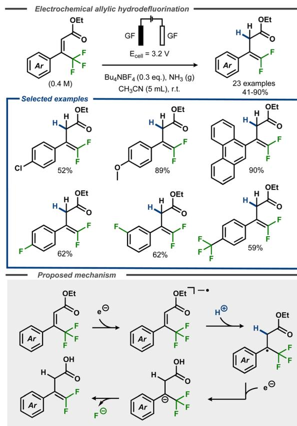
Fig. 16 Electroreductive formation of *gem*-difluorostyrenes from  $\alpha,\alpha,\alpha$ -trifluoromethyl cinnamates.<sup>62</sup>
