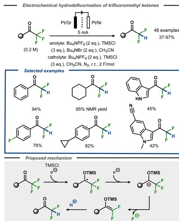
Fig. 23 Selective monoreduction of  $\alpha,\alpha,\alpha$ -trifluoromethyl ketones.<sup>77</sup>
