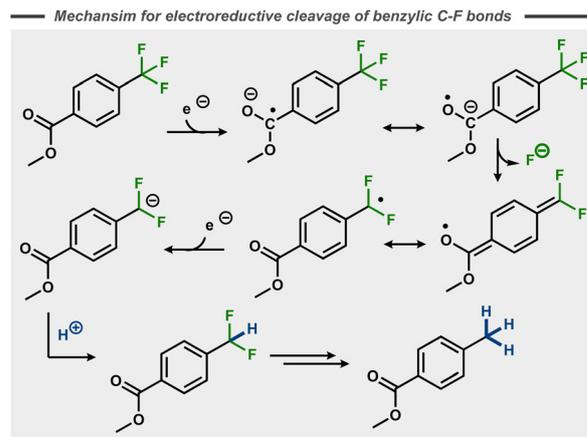
**Fig. 11** Reductive C–F bond cleavage mechanism for a trifluoromethyl arene.<sup>50</sup>
