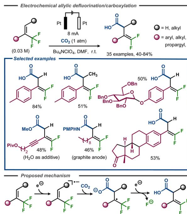
Fig. 17 Electroreductive formation of carboxylated *gem*-difluorostyrenes from  $\alpha$ -trifluoromethyl styrenes.<sup>63</sup>
