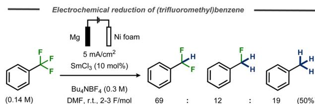
**Fig. 12** Samarium-catalyzed C–F bond cleavage in trifluoromethyl benzene.<sup>29</sup>
