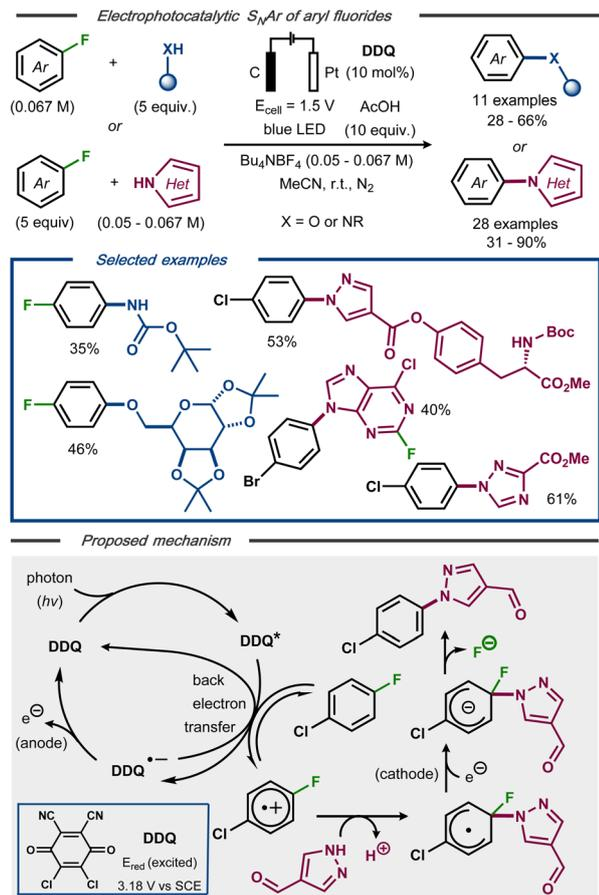
**Fig. 9** Top: Electrophotocatalytic nucleophilic aromatic substitution of aryl fluorides.<sup>46</sup> Bottom: Proposed mechanism.
