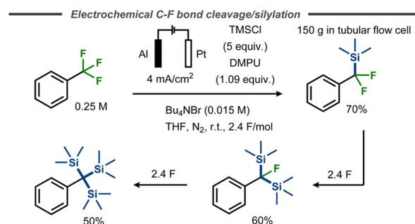
**Fig. 14** Defluorinative silylation of benzyl fluorides with TMSCl.<sup>56</sup>
