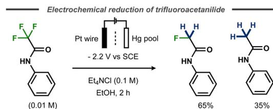
Fig. 20 Electrochemical defluorination of  $\alpha,\alpha,\alpha$ -trifluoroacetanilide.<sup>72</sup>
