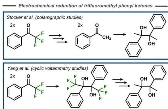
Fig. 19 Electroreductive pinacolization of  $\alpha,\alpha,\alpha$ -trifluoroacetophenone.<sup>70,71</sup>
