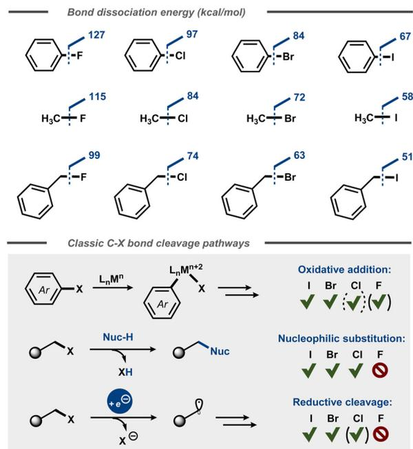
**Fig. 1** Top: Bond dissociation energies for aromatic and aliphatic C–X bonds.<sup>4</sup> Bottom: Oxidative addition, nucleophilic substitution, and reductive cleavage of C–X bonds.
