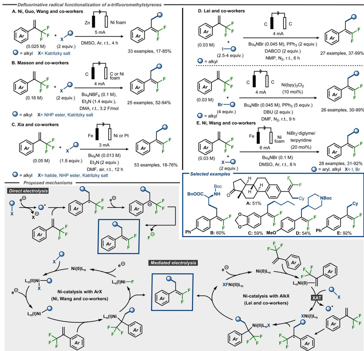
**Fig. 18** Electrocatalytic formation of  $\gamma$ -functionalized *gem*-difluorostyrenes from  $\alpha$ -trifluoromethyl styrenes and radical precursors.<sup>64–68</sup>
