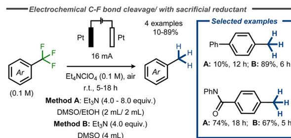
**Fig. 15** Electroreductive C–F bond cleavage in benzyl fluorides with Et<sub>3</sub>N as sacrificial reductant.<sup>60</sup>
