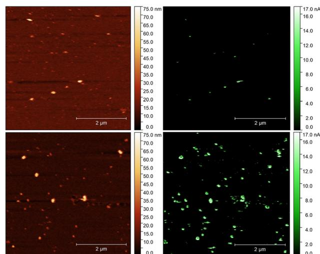
**Fig. 4** AFM (A and C) and conductive AFM (B and D) images of the NIP (A and B) and MIP (C and D) films after a 30 s electrodeposition of gold from a 0.2 mM HAuCl<sub>4</sub> solution.
