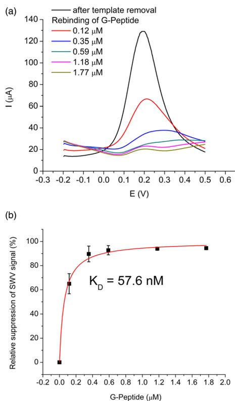
**Fig. 1** (A) SWV curves of the MIP film after template removal recorded in PBS containing 5 mM  $\text{K}_3[\text{Fe}(\text{CN})_6]/\text{K}_4[\text{Fe}(\text{CN})_6]$  upon binding G-Peptide at different concentrations as indicated. (B) The corresponding Langmuir binding isotherm of G-Peptide to the MIP. Error bars for  $n = 3$ .
