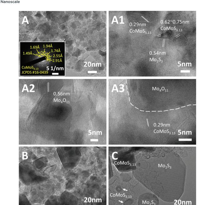
Fig. 4 TEM images of (A) CoMoS-600, (B) CoMoS-800 and (C) CoMoS-1000. The inset in (A) is the SAED pattern of CoMoS-600. (A1-A3) Are high resolution TEM images of CoMoS-600.
