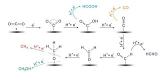
Fig. 6 The proposed reaction mechanism of production of mainly C<sub>1</sub> products by electrochemical CO2 reduction. Adapted from ref. 100. © 2017 Wiley-VCH Verlag GmbH & Co. KGaA, Weinheim.
