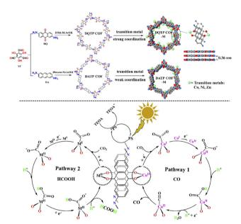
Fig. 7 Synthesis and metallization process of DQTP COF and DATP COF and proposed mechanism for the photocatalytic reduction of CO2 with DQTP-COF-M (M = Zn, Ni, and Co). Adapted from ref. 107. © 2019 Elsevier B.V. All rights reserved
