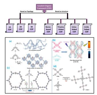
Examples of the formation of covalent organic frameworks in different dimensions. The schematic diagram for the production of (a) and (b) 1D covalent organic framework, (c) 2D COF, and (d) 3D COF. Adapted with permission from ref. 26. Copyright © 2020, The Author(s); ref. 25. Copyright © 2020 American Chemical Society; ref. 37. © 2020 Elsevier B.V. All rights reserved; and ref. 47. Copyright © 2021 American Chemical Society.
