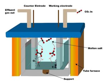
Fig. 1 Schematic of the MSCC-ET reactor.
