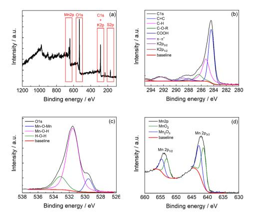
Fig. 5 (a) XPS survey spectra of C-50 and high-resolution XPS spectra of the (b) C1s region, (c) O1s region, and (d) Mn2p region.
