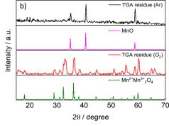
Fig. 6 (a) TGA curves of C-50 in Ar and O<sub>2</sub> at 10 °C min<sup>-1</sup>. (b) XRD patterns of the residues from the TGA of Fig. 6a, MnO (reference code 01-075-0626) and Mn<sub>3</sub>O<sub>4</sub> (reference code 01-089-4837).
